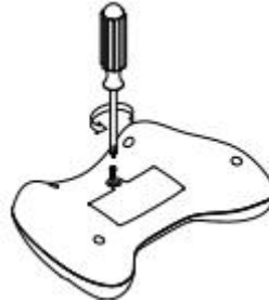
Loosen the battery cover screw
