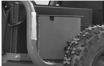
Controller & air break switch box
